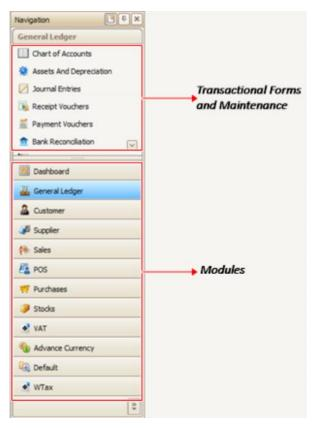
There are instances that the Navigation Pane is closed accidentally. To get it Visible, under *View* in Menu Ribbon *> Panels > Navigation > Visible*.
